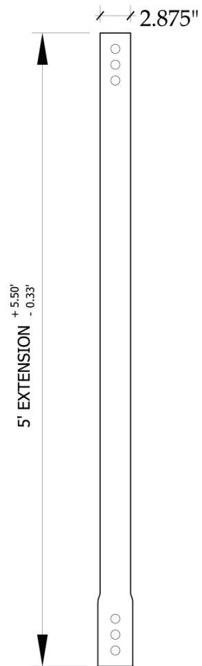
FIGURE 5—2.875-INCH DIAMETER SHAFT HELICAL PILE LEAD SECTION, EXTENSION SECTION AND HELICAL PLATES (TYPICAL)
